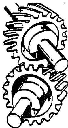
Figure 17. Crossed axis helical gears.
